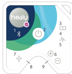
Figure 2.3.1.1: Healy top view: Pos. 1 Icon and LED for Bluetooth Connection; Pos. 2 On-Off Button; Pos. 3 Battery icon, Pos. 4 LED for generator action (if stimulator output is active, then the LED is blinking) and battery indicator; Pos. 5 Generator icon; Pos. 6 Icons for the positive and negative electrode plugs; Pos. 7 USB-Connector icon; Pos. 8 Socket for power supply
